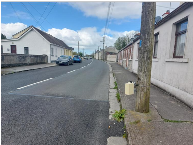
VEHICLE SPEED AND TRAFFIC VOLUME COUNTER ON OLD GALWAY ROAD, LOUGHREA TO MONITOR VOLUME AND SPEED OF TRAFFIC.
